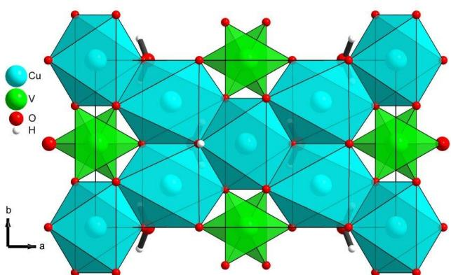
Volborthite :  $\text{Cu}_3(\text{V}_2\text{O}_7)(\text{OH})_2(\text{H}_2\text{O})_2$  [53]
