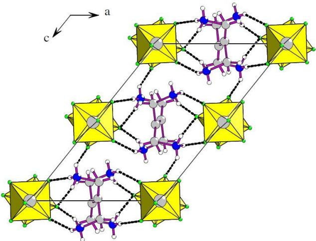
1D hybrid fluoroaluminate  $\text{C}_6\text{N}_4\text{H}_{20}\text{Al}_2\text{F}_{10}$  [149]
