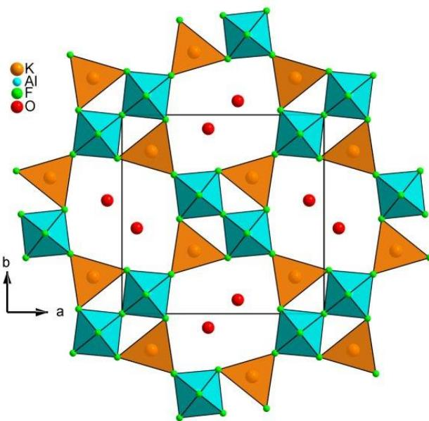
$K_2(H_5O_2)(Al_2F_9)$  obtained from a spontaneous decomposition of  $K(H_3O)_2AlF_6$  in a drawer [78]
