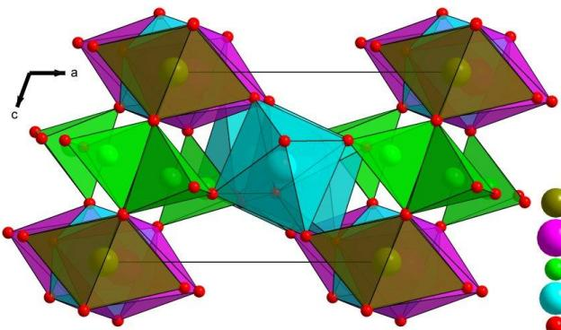
Gormanite :  $(\text{Fe}, \text{Mg})_3(\text{Al}, \text{Fe})_4(\text{PO}_4)_4(\text{OH})_6 \cdot 2\text{H}_2\text{O}$  [132]
