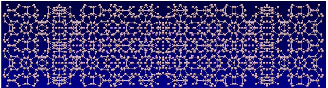
$\text{Al}_{56}(\text{Cu},\text{Zn})_{11}\text{Li}_{33}$ , close to the quasi-crystals strange world [72]
