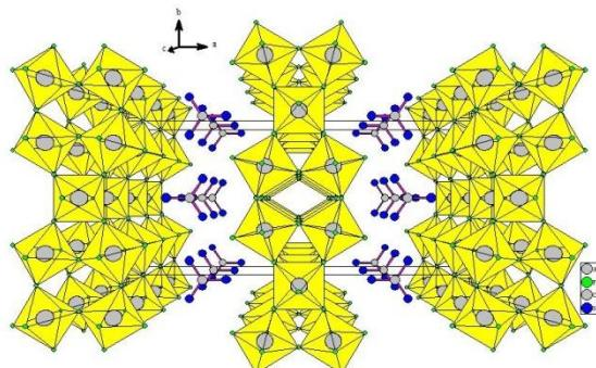
Layered hybrid fluoroaluminate C<sub>2</sub>H<sub>12</sub>Al<sub>5</sub>F<sub>17</sub>N<sub>6</sub>
